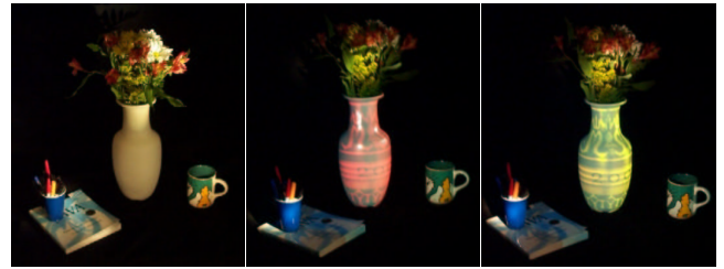
Figure 6: (Left) The underlying physical object is a white diffuse clay vase. (Middle and right) View-dependent effects, such as specular highlights, can be generated by tracking the user's location and projecting images on the physical vase.
