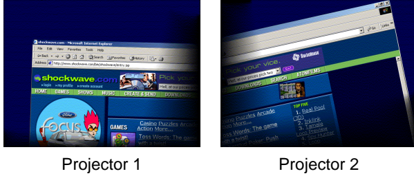
Figure 6. Rendering with pre-warping using homography and intensity blending. Note the clipped rectangle and intensity blending using alpha maps from Figure 4.
