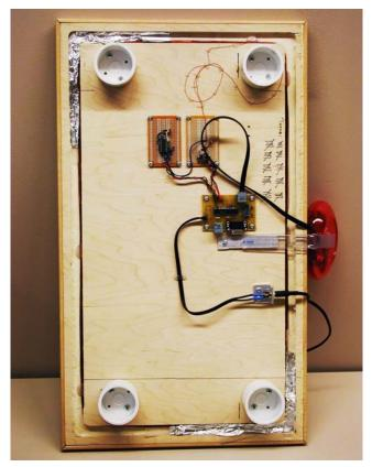
Figure 10. Underneath the iGlassware table.
