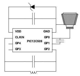
Figure 8. The iGlassware glass schematic.
