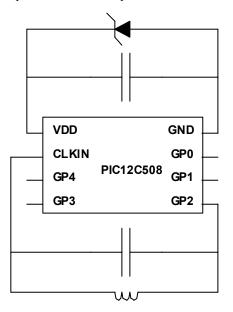
Figure 6. Ignatov's PIC-based RFID tag [6].
