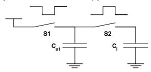
Figure 2. A Switched-capacitor "RC" circuit.
