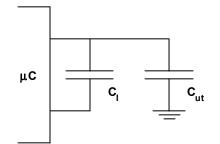
Figure 4. The microcontroller-based capacitance measurement circuit.
