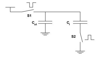
Figure 3. A Switched-capacitor "RC" circuit with S2 moved to the bottom plate.
