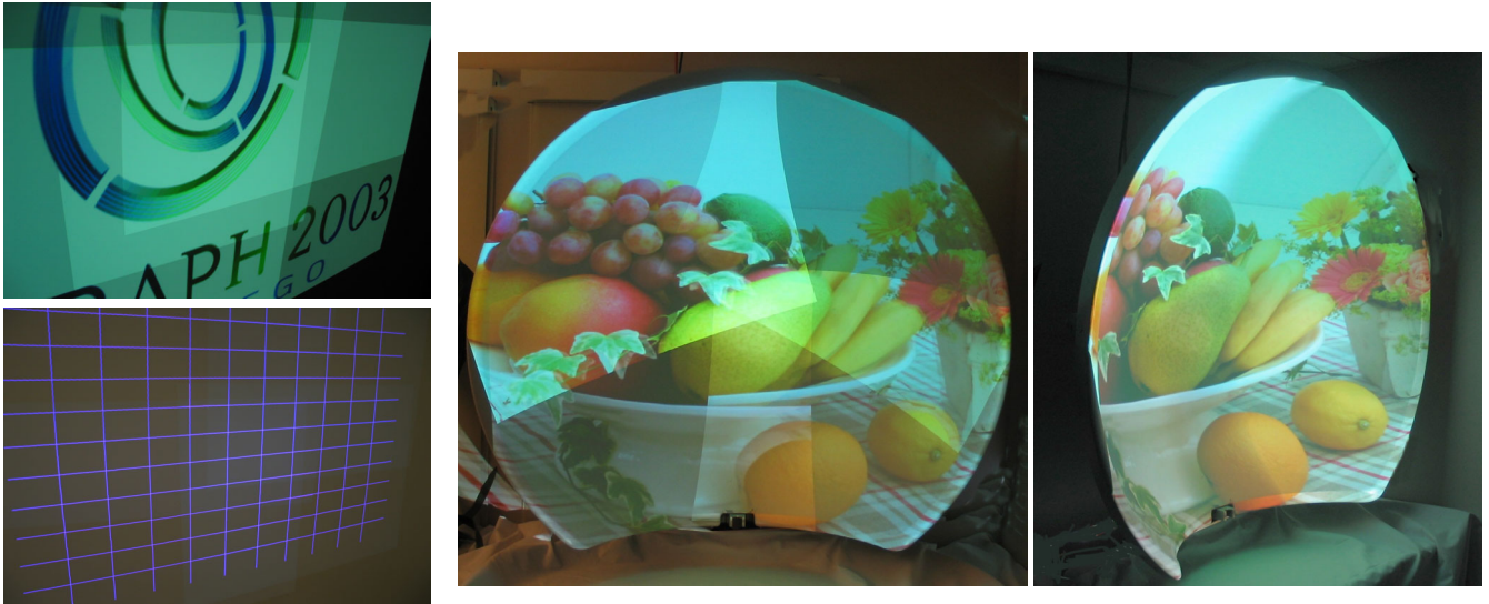
Figure 6: Left : closeup of projector overlap for a four-unit cluster in a 2x2 arrangement. Left-top : projection of ordinary images (without normalization of illumination in the overlap area); Left-bottom : a projected grid for the same configuration provides a clear visual indication that the registration after global alignment is good. Middle : four self-contained units displaying overlapping images on a spherical surface with discernible mis-registration after linear estimate of quadric transfer; Right : seamless geometrically corrected display after non-linear refinement of quadric transfer parameters and intensity normalization.
