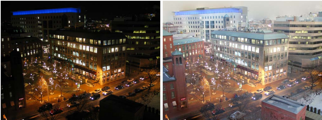
Figure 1: Automatic context enhancement of a night time scene. The image is reconstructed from a gradient field. The gradient field is a linear blend of intensity gradients of the night time image and a corresponding day time image of the same scene.
