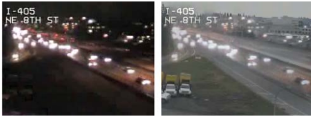
Figure 2: Enhanced traffic video. A low quality nighttime image, and a frame from the final output of our algorithm.
