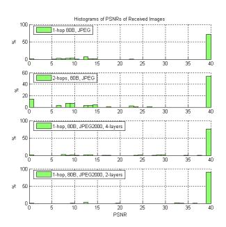
Fig. 6. The PSNR distribution of received images a) JPEG 1-hop transmission, b)JPEG 2-hop transmission, c) 4 quality layer JPEG 2000 1-hop transmission d) 2 quality layer JPEG2000 1-hop
