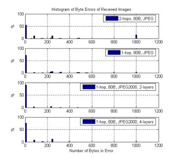
Fig. 5. Byte error histograms in two different routing cases with 80 byte application payload sizes. a) JPEG 2-hop transmission, b)JPEG 1-hop transmission, c) 2 quality layer JPEG 2000 1-hop transmission d) 4 quality layer JPEG2000 1-hop
