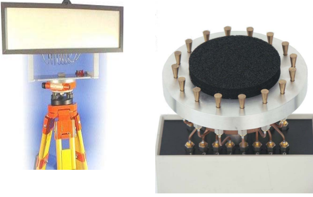
Fig. 1. An 8-element dual polarized uniform linear patch array was used at the transmit side and a 16-element vertically polarized uniform circular array was used at the receive side.
