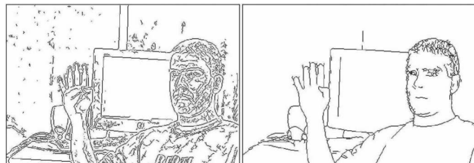
10 Cluttered scene using (a) Canny edges and (b) depth edges.
