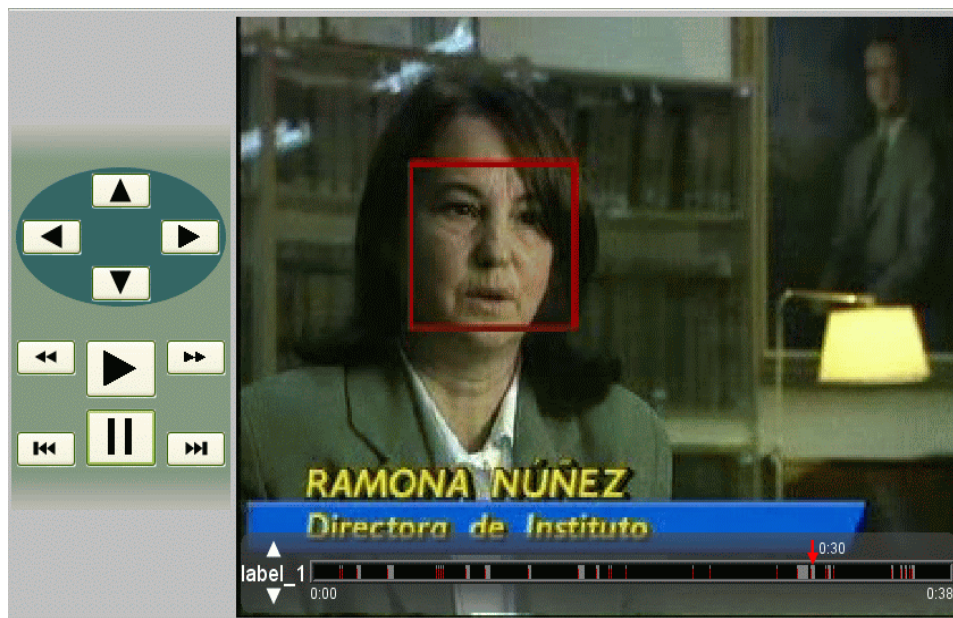
Figure 1. A screenshot of the consumer electronics video browsing interface. The user can browse through alternative summaries using up-down keys, and skip through segments or markers using the left-right keys. A time bar at the bottom shows the included segments, and the current position.
