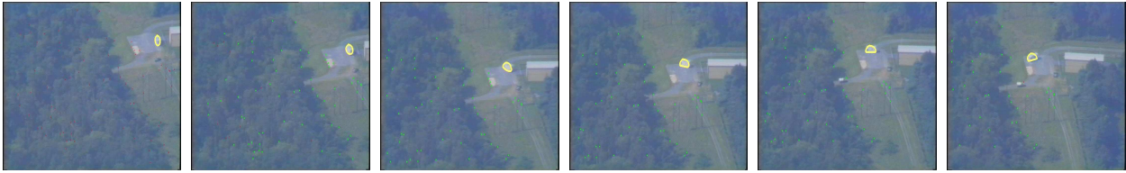
Fig. 14. An airborne sequence with a white truck moving on the ground. The truck shows a back view in frames (1) and (2), then shows the back-right view in frame (3), a side view in (4) and (5) and a front-right view in frame (6). This experiment demonstrates that the contour-based tracker can give satisfactory results on sequences containing 3D object rotations.
