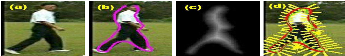
Fig. 3. An example of how to make a normal line scanning adaptive. (a) cropped original object; (b) estimated contour; (c) distance transformed object; (d) normal lines on control points.
