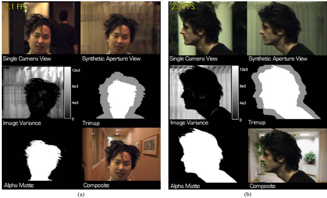
Figure 7: Alpha matting people and hair. (a) A snapshot from a video sequence of a moving head. Observe that there is a moving person in the background that is correctly segmented out in the composite. (b) A snapshot from a video sequence obtained by a moving camera array.
