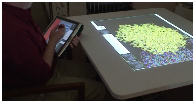
Figure 5. Selections on the tablet are reflected on the tabletop display. In this figure, one of the four chains in the protein is selected. Selected atoms appear in light yellow.
