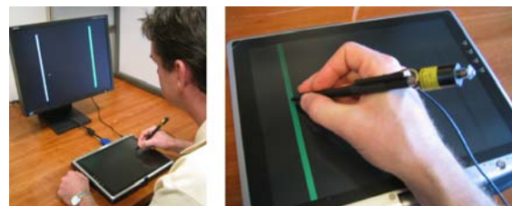
Figure 1. (left) Indirect input: stylus input and display are separated. (right) Direct input: stylus input and display are co-incident. The same tactile feedback stylus is used in both cases.
