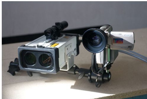
Figure 3: Laser distance meter and video camera for documentation
