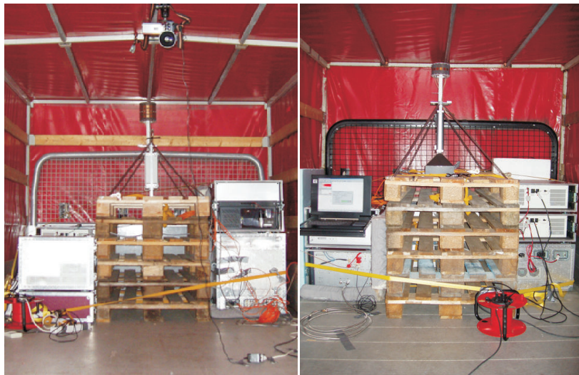
Figure 5: Loading spaces with the measurement equipment — left Rx, right Tx
