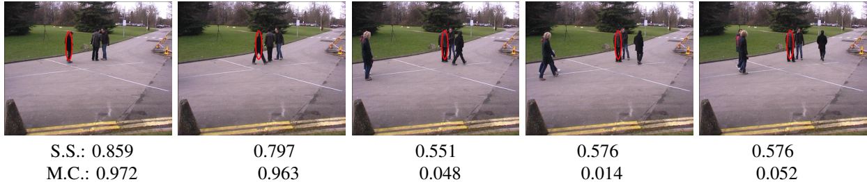
Figure 7. A person walks across another person with similar appearance. Our method detects the tracking confusion. SS represents similarity score based on color information, and MC denotes multifold consistency.
