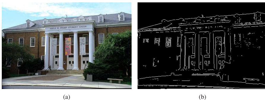
Fig. 1.1 Fitting a rectangle to an entrance. Various sources of error arise here – feature points are noisy, grouping of the points into a rectangle is a challenge, and a rectangle is not an accurate model for the entrance.
