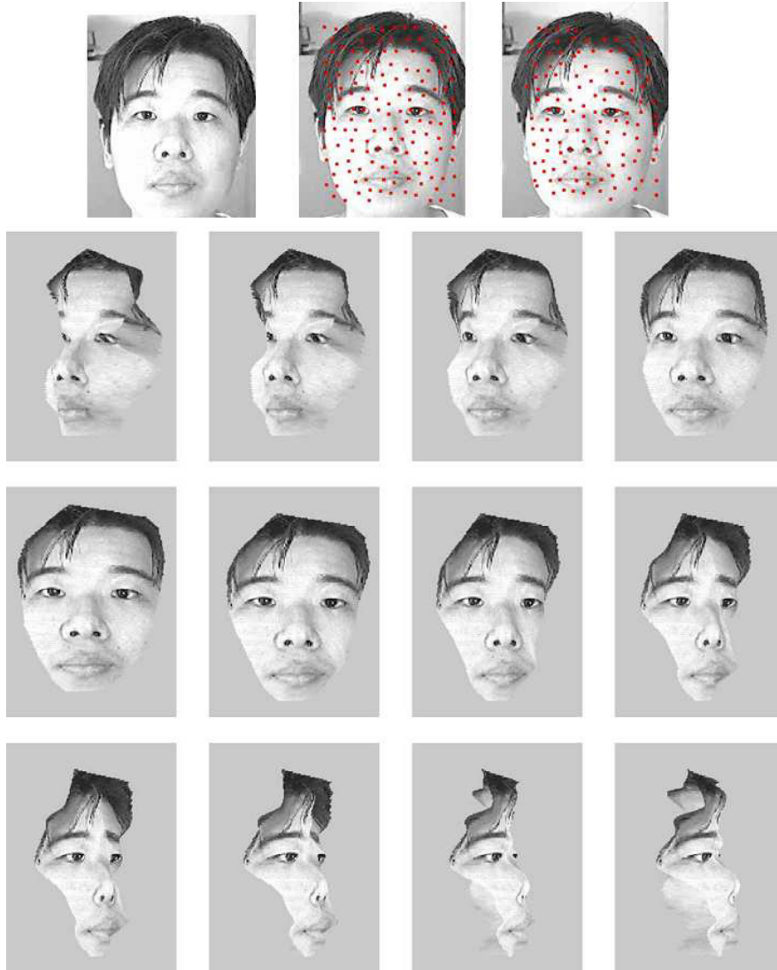
Fig. 5.3 The intensity texture map, tracked feature points on two frames, and images synthesized from the reconstructed 3D model of the face. These results were first reported in [160].
