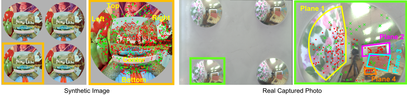
Figure 5. (Left) Synthetic image rendered with POV-Ray and zoom of a mirror image. (Right) Real captured photo and zoom of a mirror image. SIFT feature correspondences across mirror images are superimposed on the zoomed in mirror images. Red dots and green crosses respectively represent inliers and outliers determined by our iterative bundle adjustment procedure.
