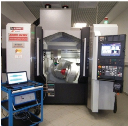
Fig. 6. : Five-axis machining center and data acquisition system used in the experimental setup to validate the feedrate scheduling strategies.
