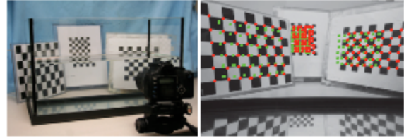
Figure 6. (Left) Setup. (Right) Photo captured by looking through a water tank. Projected 3D points are overlaid by applying pose estimated using CA (green) and our algorithm (red).
