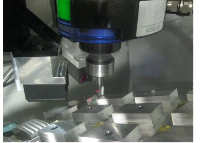
Figure 8: Experimental setup for measuring force and tool deflection
