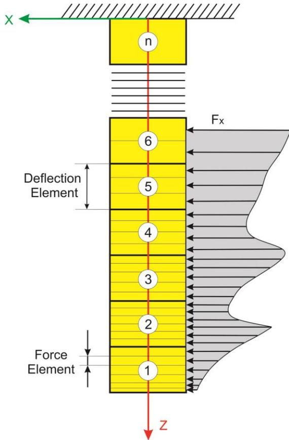
Figure 5: FEM model of tool deflection
