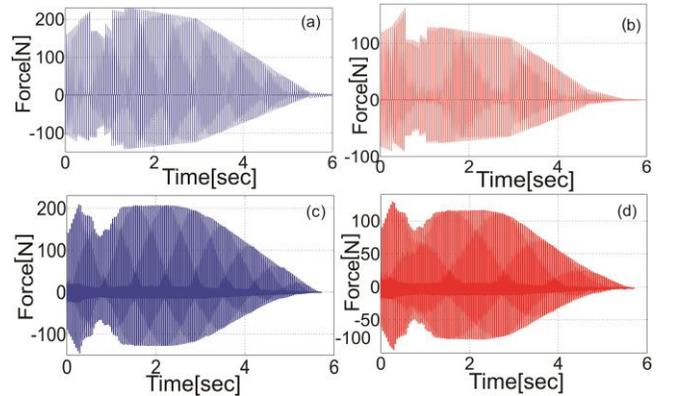
Figure 9: Simulated and measured cutting forces. (a) simulated cutting forces in y direction, (b) simulated cutting forces in x direction, (c) measured cutting forces in y direction and (d) measured cutting forces in x direction.
