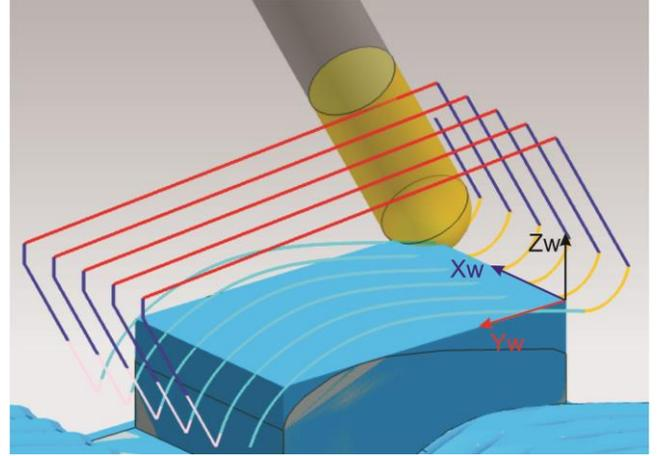
Figure 2: Cutter and workpiece geometry
