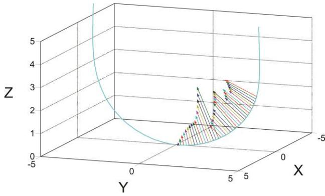
Figure 4: Distributed cutting force along cutting flute
