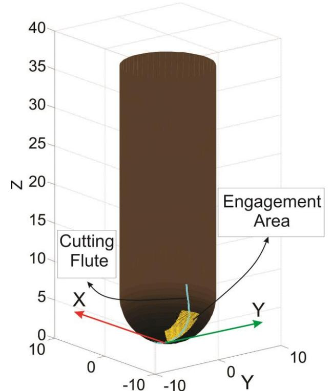
Figure 3: Modeled engagement for five-axis ball-end milling of airfoil geometry
