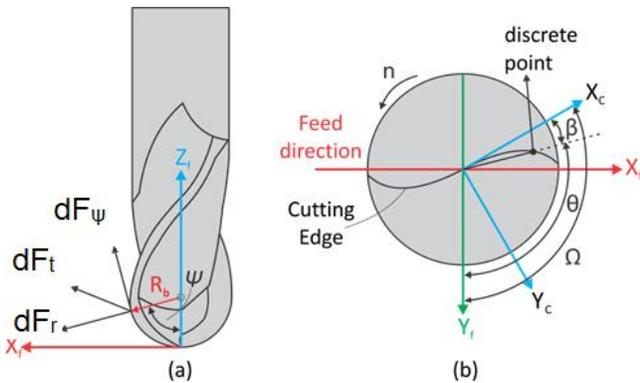
Figure 1: Illustration of cutting force vectors and cutting edge geometry
