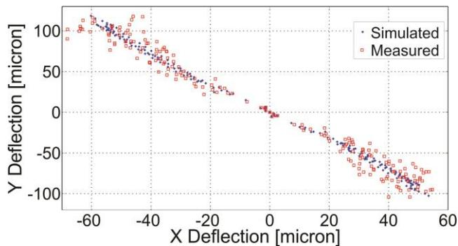
Figure 10: Simulated and measured deflection during the cutting process at the tip of the tool
