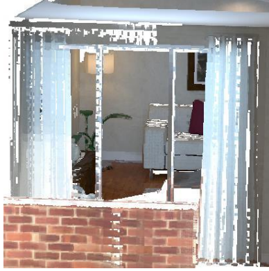
(a) Original point cloud of the window area.
