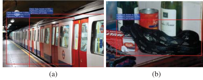
Fig. 3: Images preferred by LT/C . Top rows show two figures are two cases that will be selected by LT/C , which are images with certain category but loose bounding box (a) or images with tight bounding box but uncertain about the category (b).
