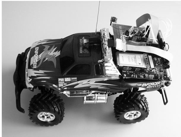
Figure 2: The prototype device mounted on a model car.
